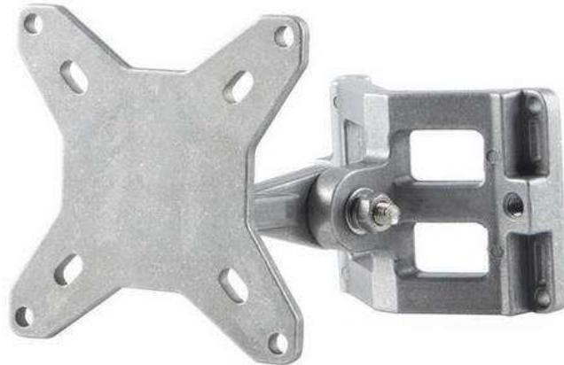
At last, it's a universal mounting bracket that is suitable for most UHF RFID antennas and mounting options, which includes mast mount and wall mount. It 's easy to mount with UDLR (up, down, left and right) adjustable clamp and tilts. There is no limit for the diameter of the mounting mast/pole. It ranges from 38mm to 100mm or more significant with optional 304 stainless steel adjustable clamps.
